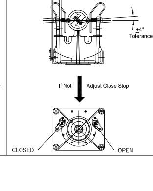
5 Check Blade Angle Blade Angle Tolerance is ± 4°
