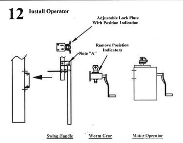
Remove 3/8" bolt to unlock swing handle. Lift handle and reinsert 3/8" bolt in open hole.
