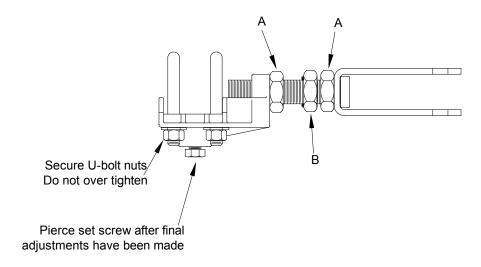
To adjust, loosen the locking nuts (A), and rotate the turning nut (B) to lengthen or shorten the offset pipe. Then tighten the locking nuts. Locking nuts must be tighten before operation.
